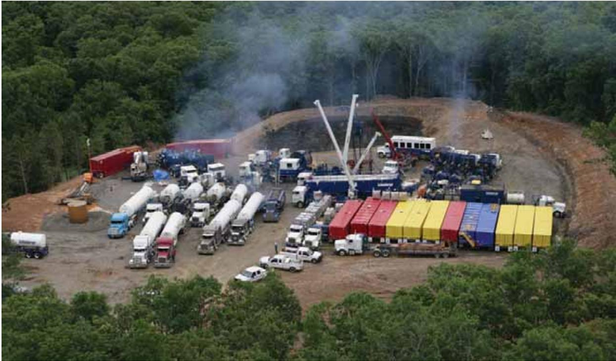
The numerous truck-mounted pumps and temporary storage tanks needed to fracture-treat the Marcellus Shale will require larger well locations. The fracturing equipment and materials on location in this photograph represent over 100 round trips to location by large tractor trailer trucks. (Photo source—Unknown)
