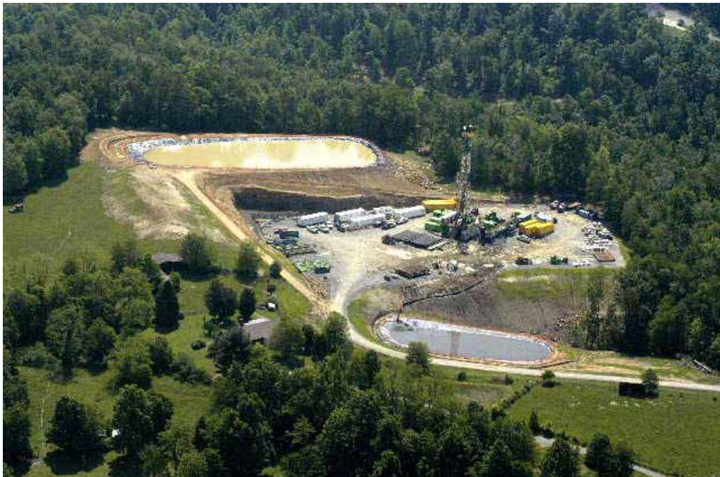
Water storage at a typical gas well (used by permission, West Virginia Surface Owners Rights Organization: www.wvsoro.org )
